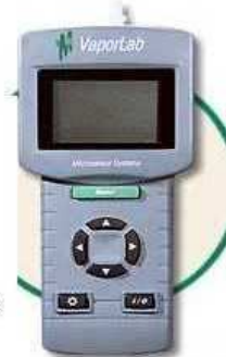
MSI Vaporlab; hand-held SAW sensor array.
